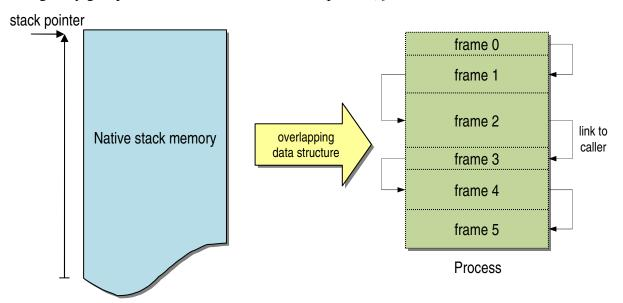
As shown in the illustration the execution stack is divided into consecutive frames, which are data structures linking the activation of a method with that of its *caller* and *callee*. Stack frames are described in [1]. The structure of stack frames in a *Digitalk* VM can be understood by browsing the class Process.
